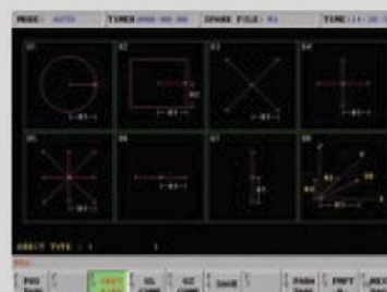
The orbital eroding function provides various orbital eroding modes. In addition to standard eroding modes, this function also provides complicated and advanced orbital eroding modes. When combining with the path return function of the controller, the machine can perform complicated inside chamfering operation.
