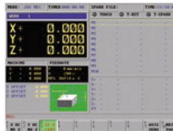
The display provides convenient touch point function by automatic and manual modes, and 50 sets of touch point memory. The edge-search values are automatically memorized into machining programs.
